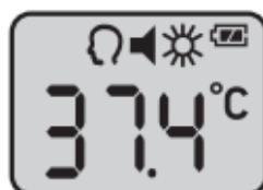
When temperature reaches 37.4 °C (or below), green backlight will turn on.
