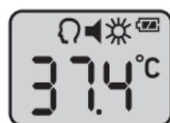
When temperature reaches  $37.5^{\circ}\text{C}$  (or higher), red backlight will turn on.
