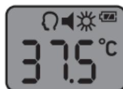
When temperature reaches 37.5 °C (or higher), red backlight will turn on.
