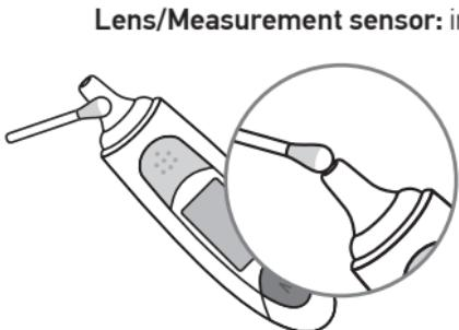
**Lens/Measurement sensor:** in case of contamination of the infrared thermometer sensor lens, the readings begin to change immediately as something interferes with the measurement (usually the readings are too low). To eliminate this problem, it is enough to wipe the sensor with a soft lint-free cloth (or cotton swab) moistened with disinfectant solution. Then it is necessary to wipe the lens with a dry soft lint-free cloth. After the cleaning procedure,
