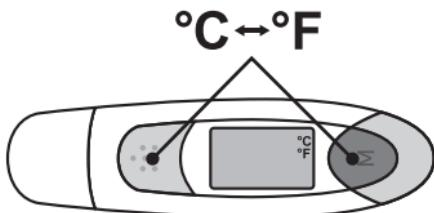
This thermometer can display result in either degrees Celsius ( $^{\circ}\text{C}$ ) or degrees Fahrenheit ( $^{\circ}\text{F}$ ).
