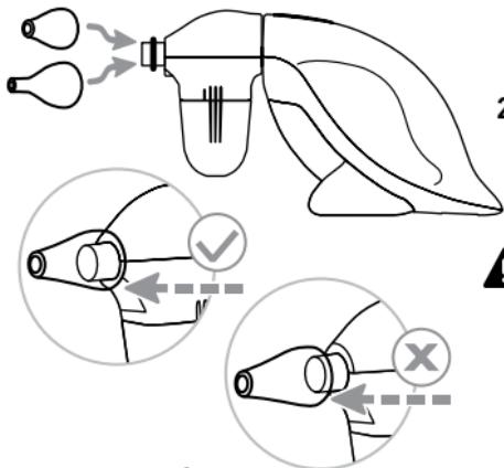
2. Be sure to place the Tip securely on the aspirator. Make sure the Tip is completely covering the rib before using.
